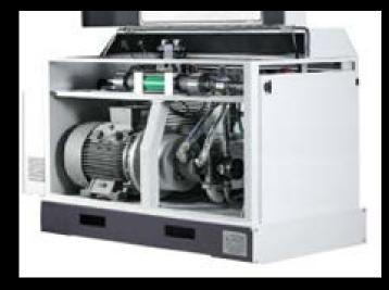
On the pump unit you will be able to get feedback from gauges such as: Oil pressure, Temperature, Inlet water pressure, high pressure, and the air inlet pressure is provided by a gauge next to the front pendant. The cutting head is Dia-line; the head body and a laser indicator allow the operator to visualise the cutting edge and calibrate the slab on the table before cutting.
