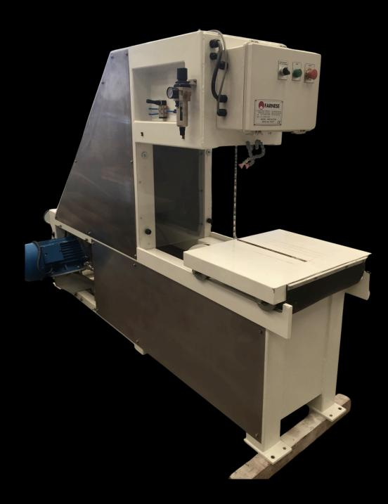
The WIRE SLITTER has been conceived for small block cutting and producing quoins from sandstone.
